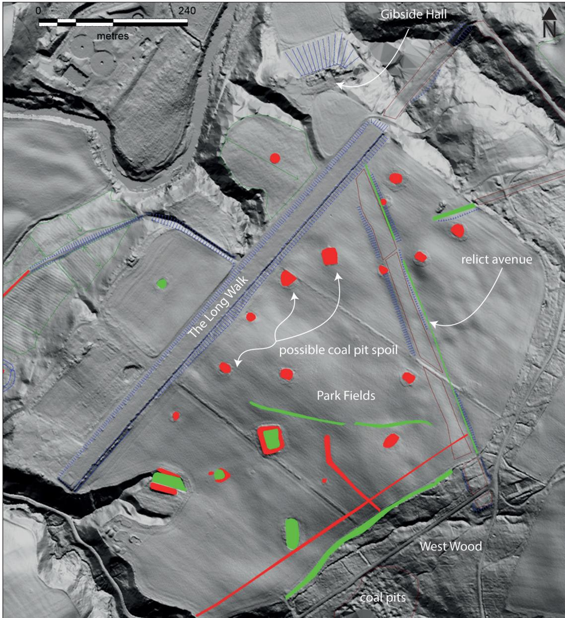
Figure 27: Landscape features and possible coal workings at Gibside. [background lidar DTM 2018 © Historic England; source Environment Agency]
