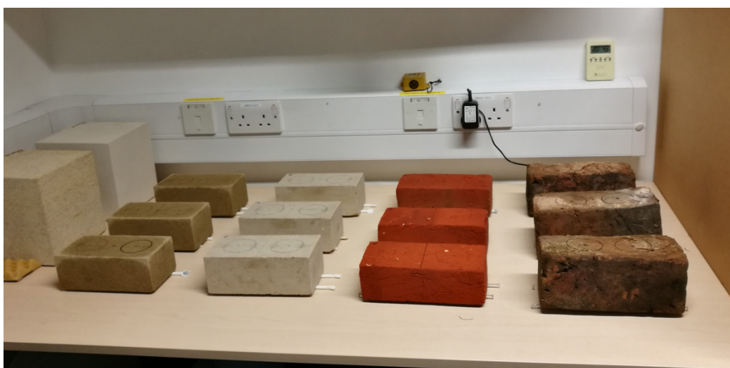
Figure 9: Blocks in place for drying tests (four material types, three replicates).
