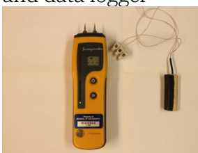
Protimeter with Historic England probe wooden dowel
