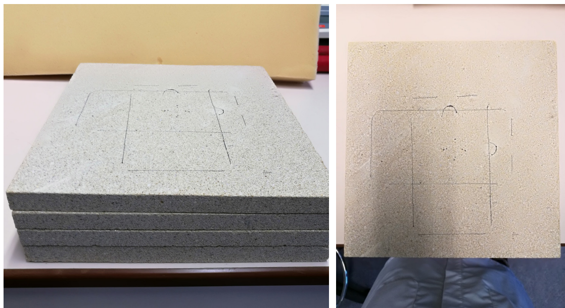
Fig 14: The Stoke Hall sandstone samples used to investigate the depth penetration of the Tramex and the Extech, showing a stack of stone slices (left) and the templates for the meters (right).
