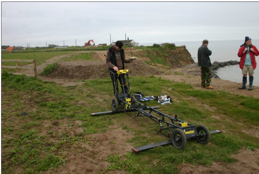
Figure 13 Using Ground Penetrating Radar on the cliff top above Happisburgh Site 1. Photo by Martin Bates.
