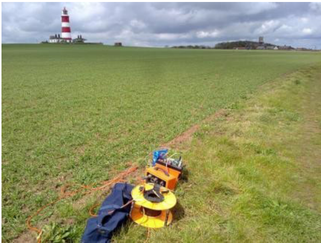
Figure A2.2 DC ABEM Terrameter resistivity meter on cliff top near Happisburgh.
