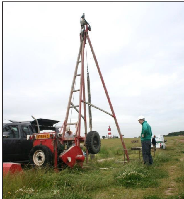
Figure 10 Using the cable percussion drilling rig on the cliff top above Happisburgh Site 1. Photo by Peter Hoare.
