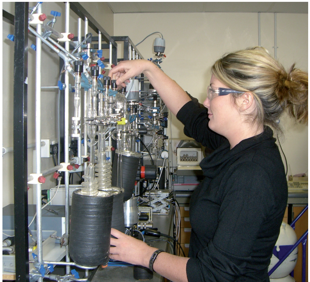
Figure 3: Combusting a sample to carbon dioxide, before its conversion into graphite for measurement by Accelerator Mass Spectrometry (photograph by H. Granlund Marsden).
