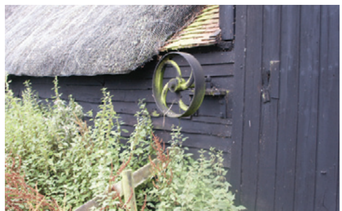
Flywheels and drive shafts for transferring the power from portable engines often provide the only indication of their use. Photo © Bob Edwards
