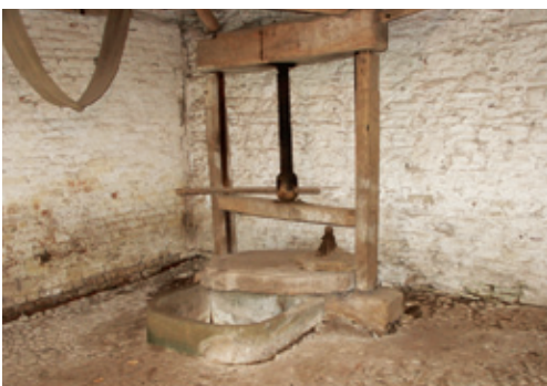
A cider press, for squeezing the juice from fruit crushed in the mill. © Jeremy Lake
