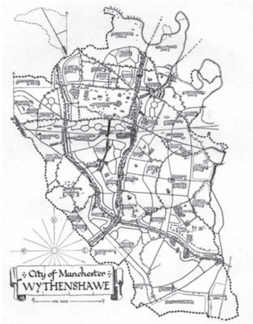
Figure 89 Barry Parker's 1931 plan for Wythenshawe featured sophisticated neighbourhood planning and landscaped parkways, influenced by American practice. [Macfadyen 1933 Fold Plan, 122]
