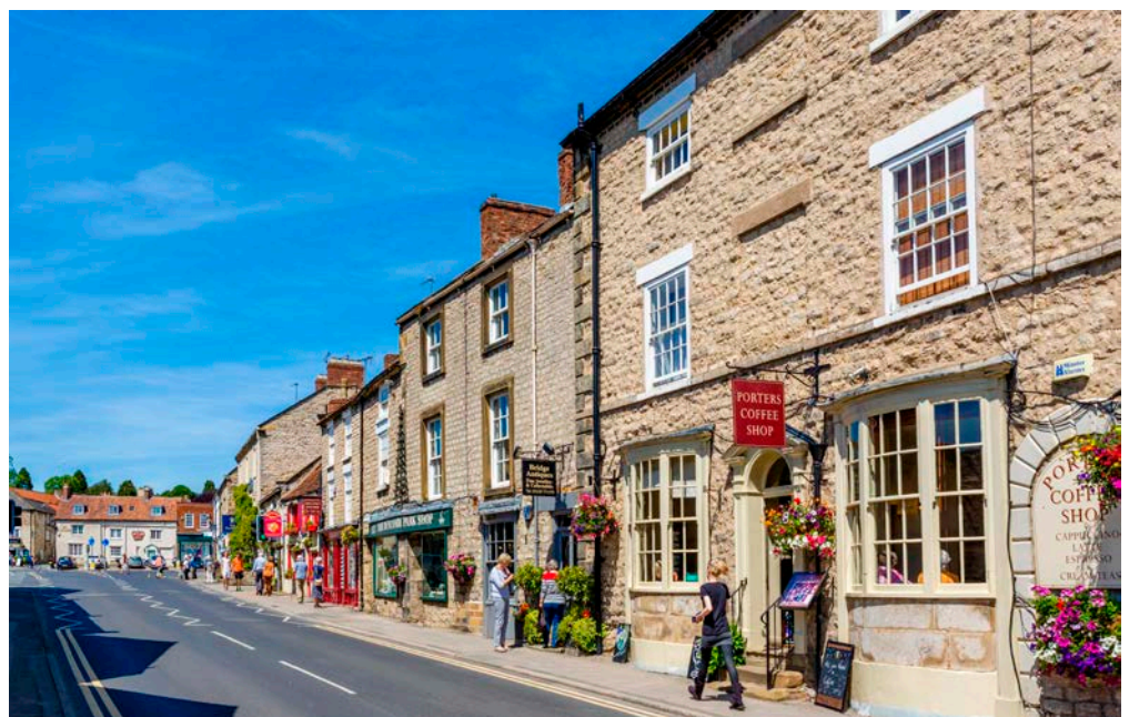
Figure 19: Bridge Street, Helmsley. Hambleton Oolite.
